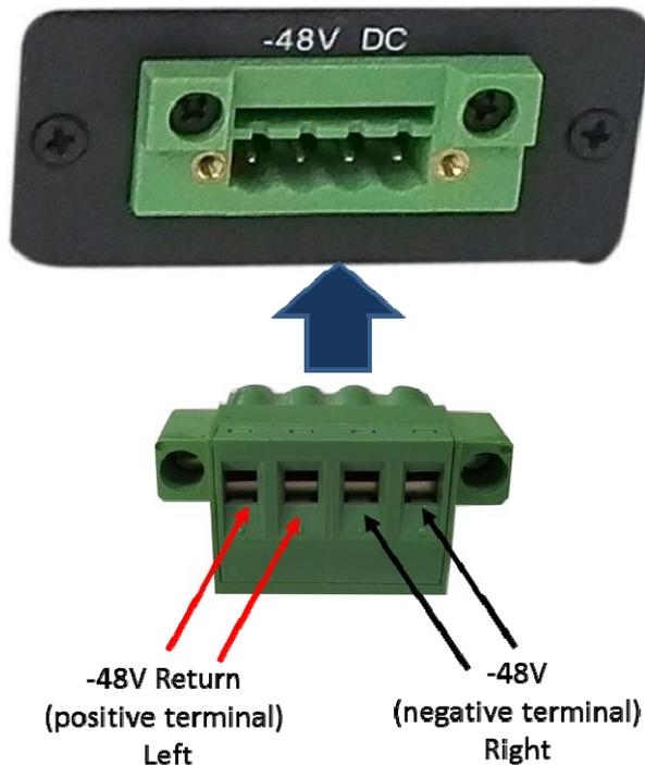
7. Repeat Step 5 and Step 7 for the other two wires to complete the assembly of the DC input power cable.
