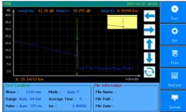
Fig.3-6 Reflection loss test
