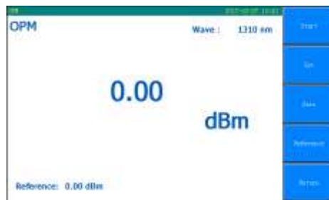
Fig.4-1 Optical power meter test interface
