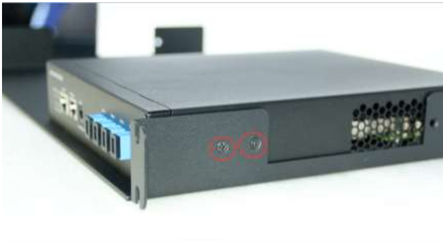
Figure 0-5 Install BD-2GPON-OEO on Tray Bracket
