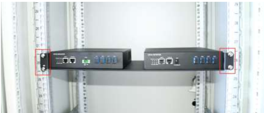
Figure 0-6 Install Tray Bracket in Cabinet
