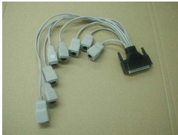
Fig. A-2-3 DB37F-RJ48C-8E1 cable adapter
