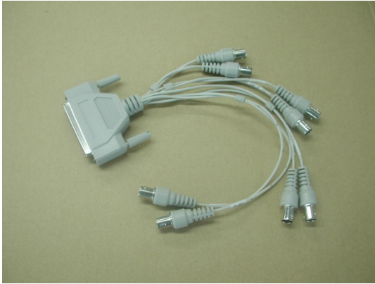
Fig. A-2-1 DB37F-BNC-4E1 cable adapter
