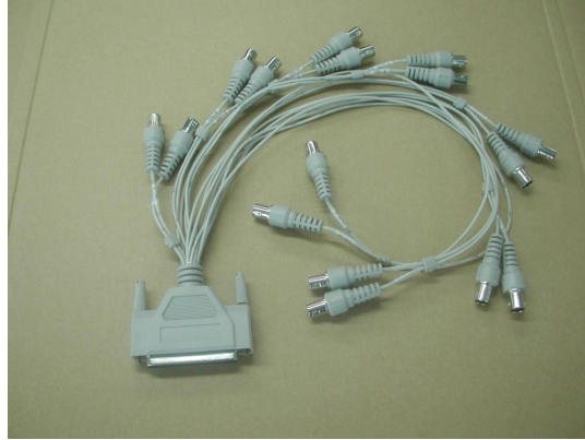
Fig. A-2-2 DB37F-BNC-8E1 cable adapter
